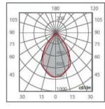
Symmetric optic for indoor lighting, elliptic emission
