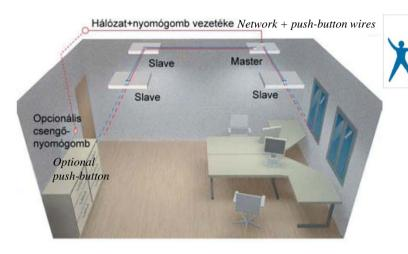
The Greenpack control system takes advantage of natural daylight, and if no one is in the room, turns off the lights.
