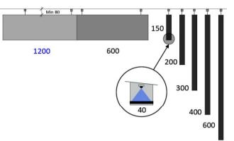
Standard colour: White RAL 9016; any RAL or NCS-Code available to order Diffuser: Opal with 72% light transmission or low brightness micro prismatic (MPS) CRI Colour Rendering Index: <83 Light Colour: 3000 K, 4000 K Suspension: Wire; rod available to special order Lumen output (4000 K): 600 mm /12 W: 1,200 lm; 900 mm / 18 W: 1,910 lm; 1,200 mm / 25 W: 2,630 lm; 1,500 mm / 32 W: 3,340 lm Mass: approx. 4.5 kg LED power: 10 W, 16 W, 22 W, 28 W, Protection class: I Dimmable DALI available to order
