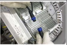
2. Disconnect the driver from the connector to modules.
