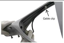
2. Put the wire through cable clip and the threading hole of Y bracket.
