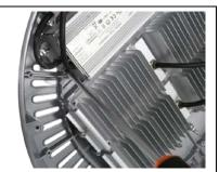
3. Unscrew the screws at ends of the driver.
