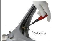
3. Tighten up the M4×12 screws on the cable clip near the threading hole.
