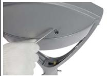
Close the cover. Then fasten the screws.Maintenance finished.
