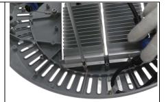
3. Unscrew the two M4x10 screws at the ends of the failed module.
