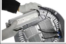
4. Replace the failed driver with a new one.
