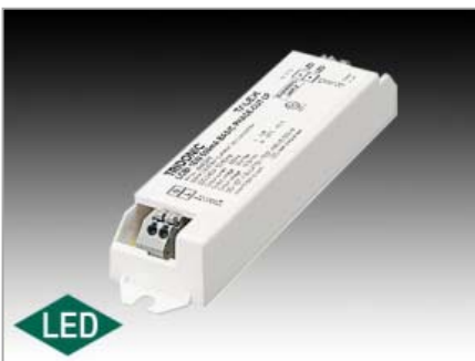
LCBI...BASIC Ip LCBI 15W 350mA BASIC Ip – LED-meghajtó, 230V, 50Hz, 21-46V, 350mA, max.16W 2-20-11-0081
